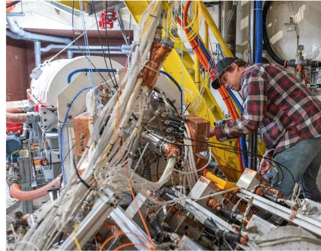
magniX propulsion system under test at NASA NEAT facility – aHV delivered partial discharge test capability
